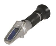
The **VIPER** Refractometer, Part No. 5026, features Automatic Temperature Compensation, dual scales for ethylene glycol and propylene glycol, a high contrast lens for easy viewing and a rugged steel body construction for durability.
